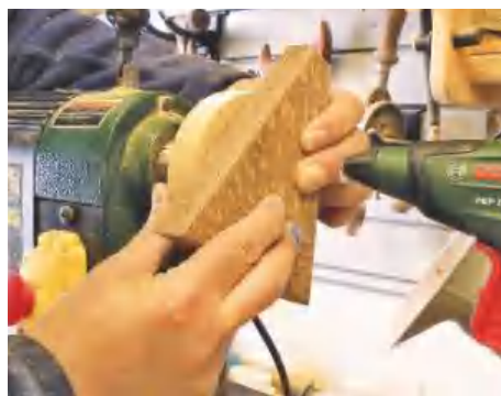
Hot melt glue on an MDF backer screwed to a faceplate holds the blank securely
